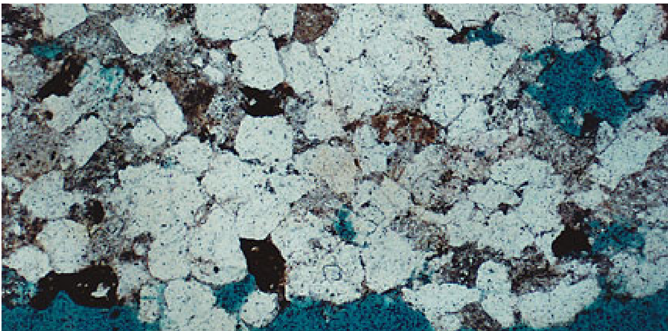
Tight gas sandstone : (voids in blue).
