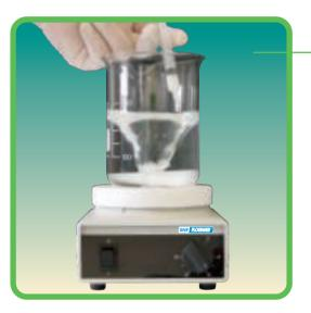
The emulsion is injected into the vortex created by the agitation. In addition, the entire amount of the emulsion should be added as quickly as possible.
