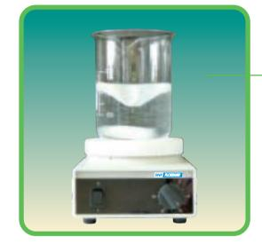
After addition of the solid, the particles, as they become hydrated, tend to swell and become translucent. The vortex closes following the increase in the viscosity.
