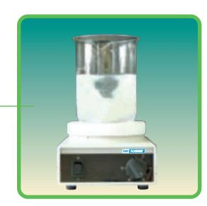
After injection, the vortex closes following the increase of viscosity of the solution (See paragraph 3.2: representation of an inversion)
