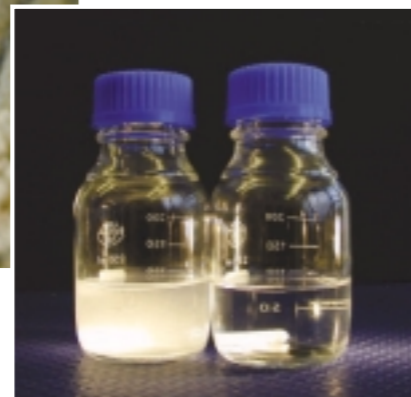
Struvite (Magnesium-Ammonium-Phosphate) in combination with sludge/polymer deposits.
