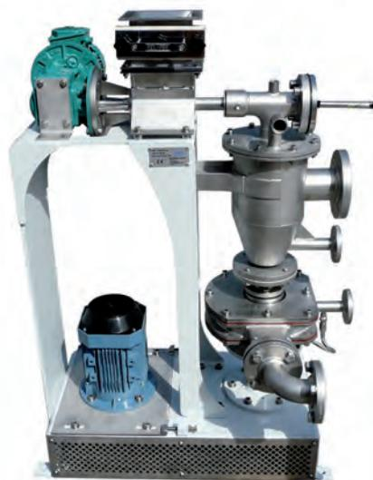
View of the Powder Hopper and FLOQUIP PSU 100 assembly
